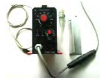
Capacity 17 ml/min Max. pressure 10 kgf/cm 2 Stroke rate 2-120 spm Voltage 220 V Current 0,61 A Power consumption 14,5 W Frequency 50/60 Hz Thermally protected
